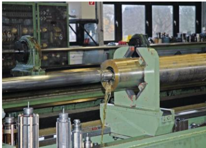
Deep Hole drilling Application
