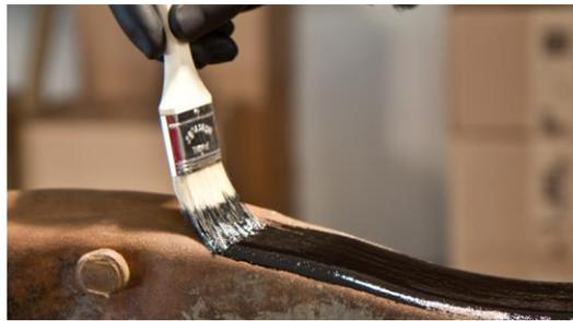
Applied by immersion, brush, swab or spray for protecting metal sheets.
